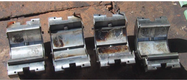
Figure 2: Damage to white metal
