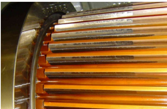
Figure 5: Damage to the teeth after refurbished bearing failure
