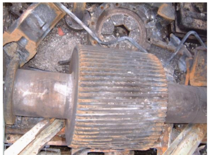
Figure 7: Total destruction of the gearbox
